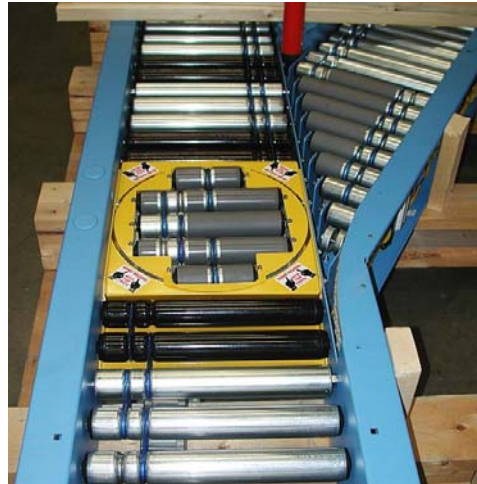
RIGHT-HAND TURNTABLE DIVERTER CONVEYOR
